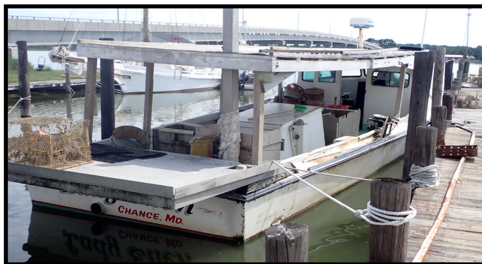
Figure 3. A starboard quarter aspect showing LADY ELLEN's low bulwarks and lack of perimeter railing or courses. The photo was taken by the attending U.S. Coast Guard Investigating Officer on 23Jul2024 at Corbin's Seafood dock in Chance, MD.
